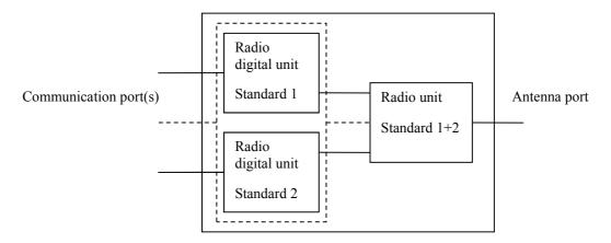
Figure 2: Multi-standard-radio equipment
